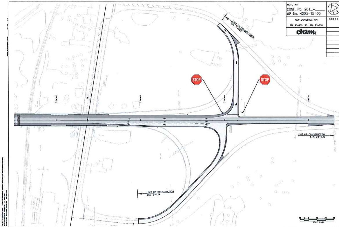
Figure 5: T-intersection with Stop Condition (Preferred Alternative)
